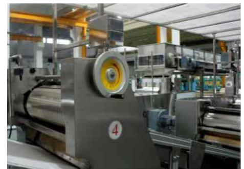
Monitor the rolling pressure and prevent metal materials entering into roller and slit to keep equipments and staff safe.
