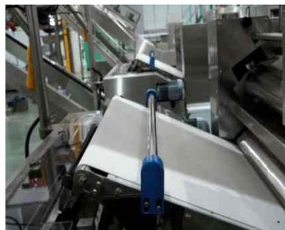
Use 100 GS magnetic rod, effectively adsorb iron materials which may enter and damage slit.
