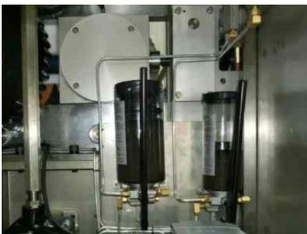
Equip with concentrated lubricating system to ensure inject lube for every lubricating spot. Simple and quick maintenance with high efficiency.
